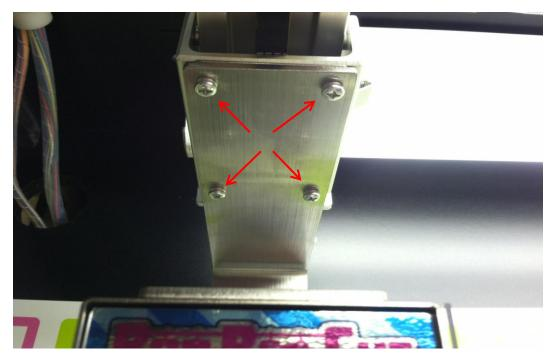
3. Loosen 4 screws holding belt in place.
