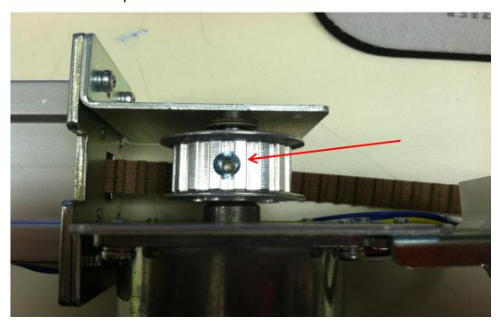
5. Remove 4 screws holding motor in place and motor should slide right out.
