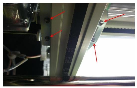
2. Remove 4 screws holding scissor assembly in place.
