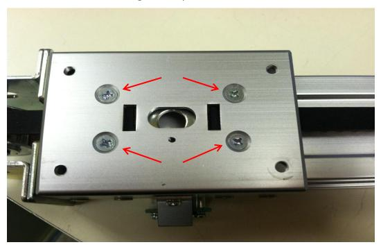
4. Loosen "Set Screw" on sprocket carefully with "2mm Allen Wrench" making sure not to strip screw.
