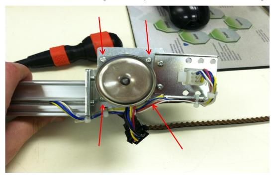
6. If "Set Screw" is too hard to loosen on sprocket and think it might be easier to get out with motor assembly off the Y-Rail, remove 2 screws holding motor assembly in place. Unscrew 1 screw with Phillips Head screwdriver and the other with long needle nose pliers.
