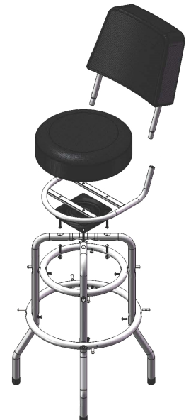
Step 4: Place the seat base on top of the swivel plate. Align the holes and insert the bolts. Screw on nuts securely with allen wrenches.
